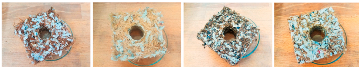
Fig. 8. Bio-briquette samples produced from various feedstock mixtures: a) CF (1:1), b) BS (1:1), c) PL (1:1), d) SB (1:1).
