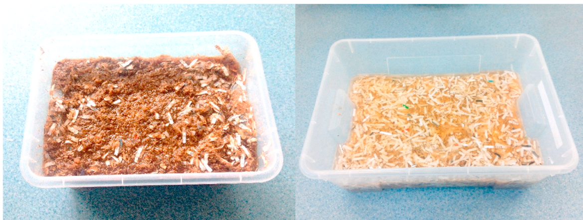
Fig. 3. Prepared feedstock mixtures: a) coconut fibre (2:1), b) bamboo skin (1:1).
