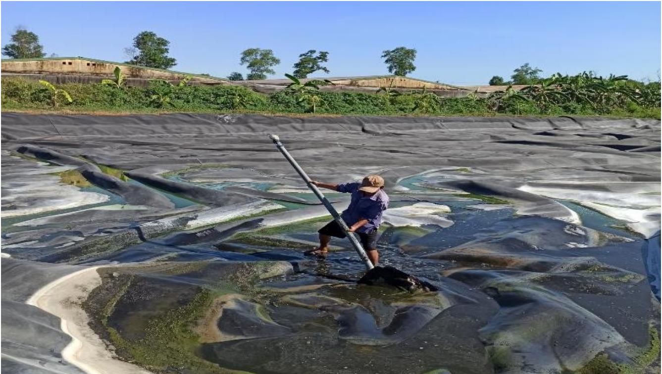
Solid biogas digestate sampling at a large-scale biogas plant at the University of Agriculture and Forestry, Hue University, Huong Tra, Thua Thien Hue, Vietnam.
